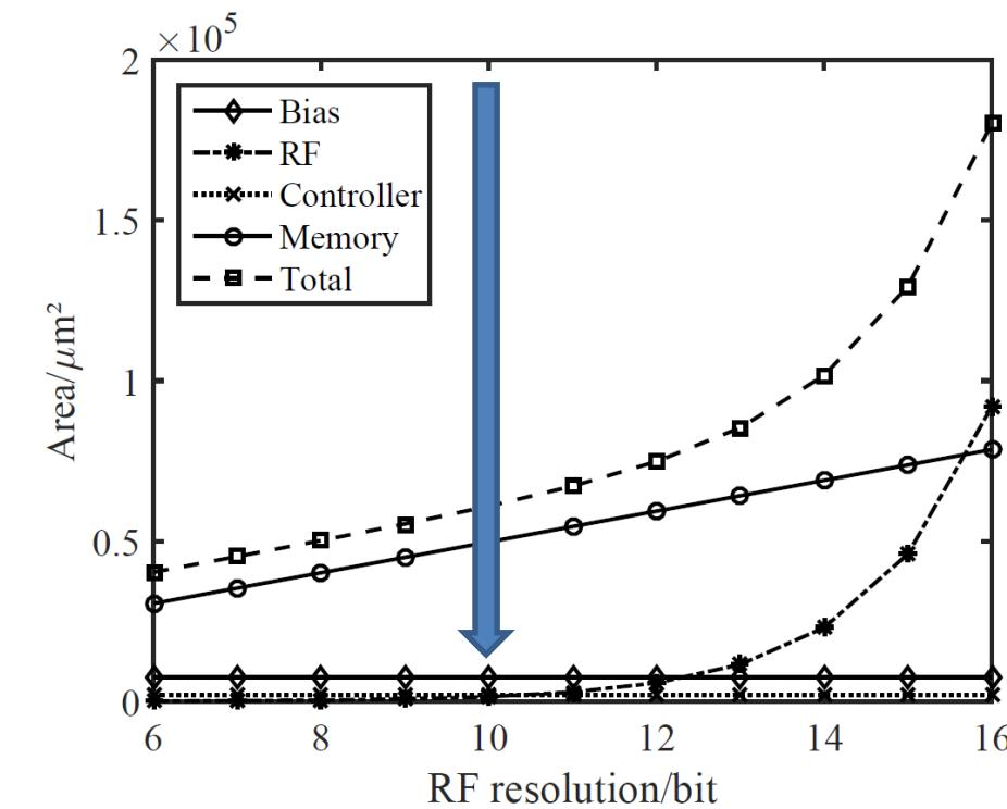
Approx. 60000  $\mu\text{m}^2$  (250 x 250  $\mu\text{m}^2$ ) control electronics for one qubit
