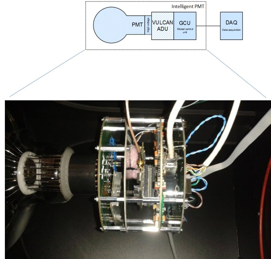
*Electronics connected to the base of PMT<sub>[5]</sub>*
