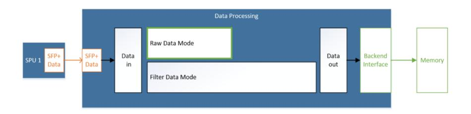
All the Data is transmitted over the Backend Interface and stored into an external Memory. a. k. a. **debugging mode**
