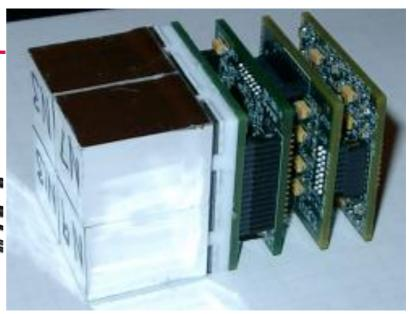
PET module is comprised of detector staks. Communication via optical link. Air cooled. Carbon shielded [2].
