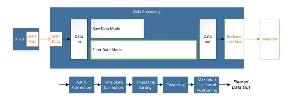
Different Filters and Algorithms reduce the Data and only the useable data for Imaging Reconstruction get transmitted over the Backend Interface and stored into an external Memory.
