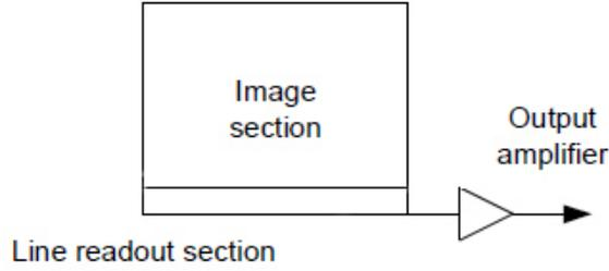
Figure 11: Typical CCD schematic.
