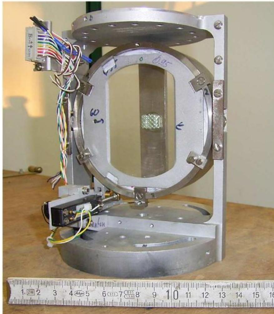
Figure 9: Crystal support with crystal and aperture of 60 mm width. On the bottom left side the servomotor with linear potentiometer for tilting of the mirror is shown (from [3]).
